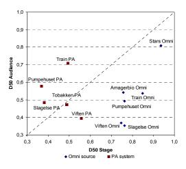
Figure 4. D50 (63-250 Hz) for audience and stage area measured with PA and omni source.
