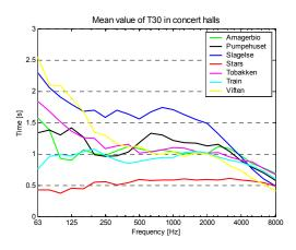
Figure 2. Position averaged T30 per 1/3 octave in all halls. NB: Tobakken and Viften were measured with PA.
