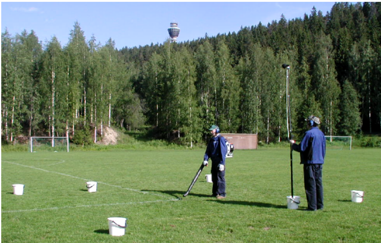
Figure 2. Leaf blower noise emission test site. Microphone positions are marked with white buckets.
