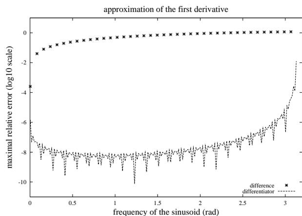
Figure 1: Maximal estimation error when approximating the (first) derivative of a sinusoid using the order-1023 differentiator. The error is acceptable for all but very high frequencies. As a comparison, the error obtained with the classic difference approximation (equivalent to choosing  $\epsilon = 1/F_s$  in the expression of Equation (23)) is plotted with stars \*.
