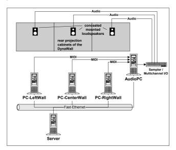
Figure 4: Hardware setup of the DynaWall
