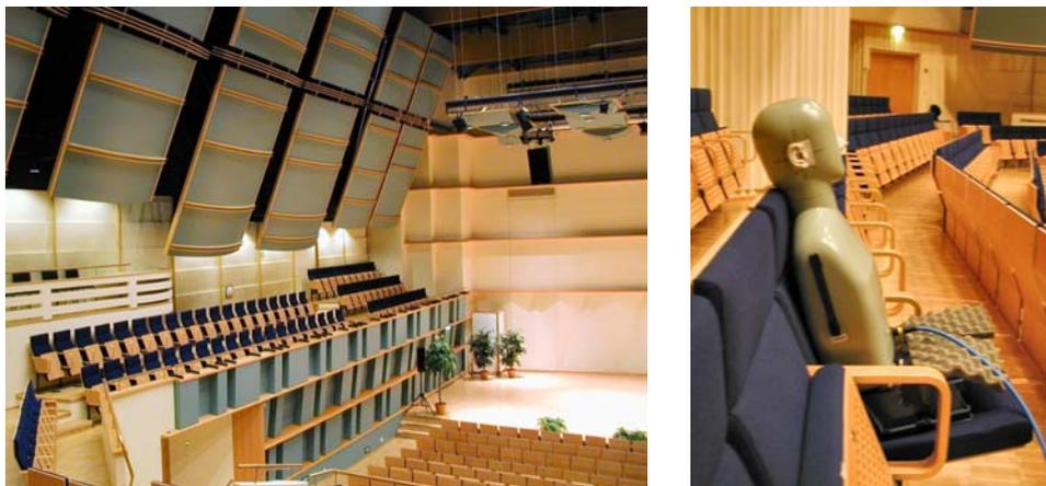
Figure 4: A view on the side of the hall (left panel) and the dummy head and torso placed on a seat for measurements (right panel).
