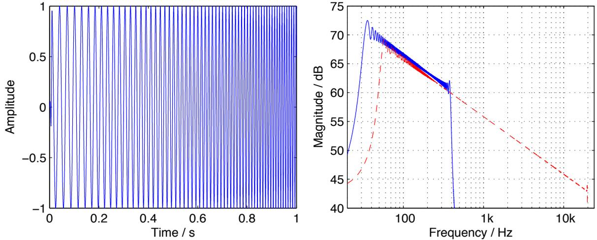
Figure 6: Left panel: Time-domain plot of the first second of the subwoofer sweep. Right panel: Magnitude spectra of the excitation signals for the subwoofer (solid line) and the omnidirectional speaker (dashed line).
