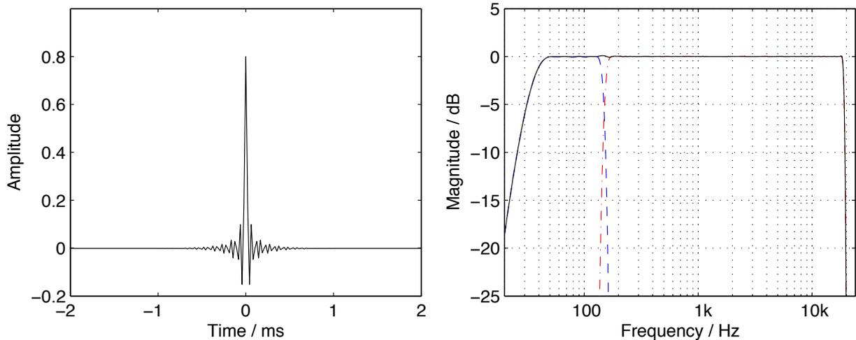
Figure 7: Left panel: Time domain impulse response of the excitation signals after deconvolution, cross-over and summation. Right panel: Magnitude spectra of the individual excitation signals after deconvolution and cross-over (subwoofer = dashed line, omnidirectional speaker = dash-dotted line), as well as the sum of the two previous responses (solid line).
