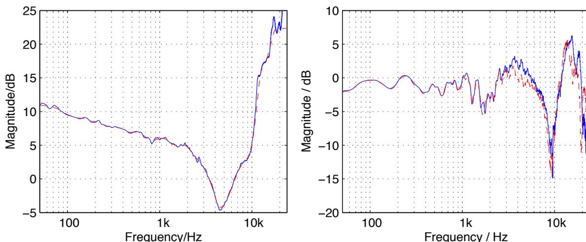
Figure 9: Left panel: Inverse diffuse field response of the dummy head (solid line) and the designed diffuse field equalization filter (dashed line). Right panel: Left (solid line) and right (dashed line) frontal HRTFs of the dummy head after diffuse field equalization.
