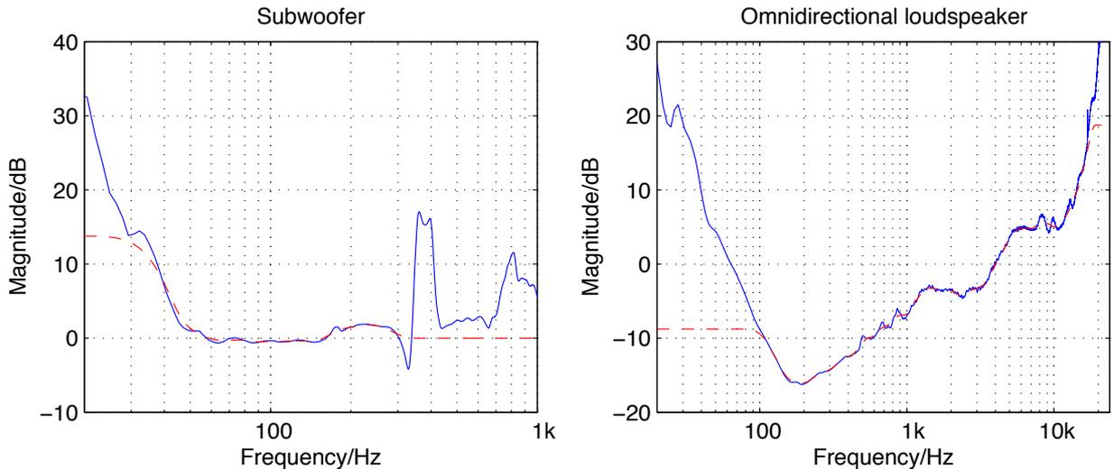
Figure 8: Inverse power responses of the sound sources (solid lines) and the magnitude responses of the compensation filters (dashed lines).
