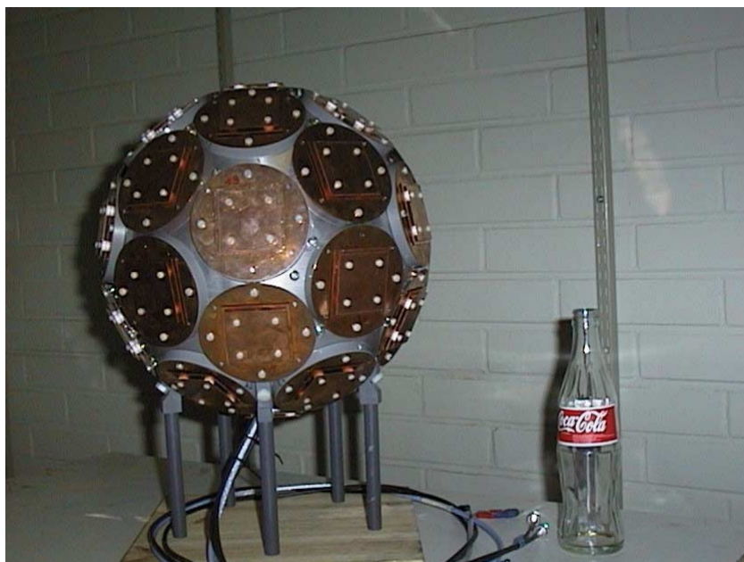
Figure 3. Spherical array of 32 dual-polarized microstrip patch elements.
