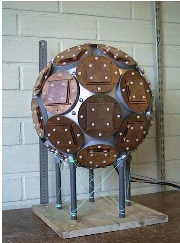
Figure 1. Spherical array of 32 dual-polarized microstrip patch elements.
