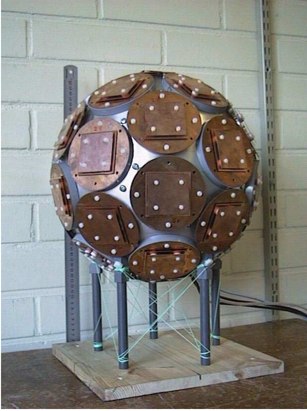
Figure 2. Spherical array of 32 dual-polarized microstrip patch elements.
