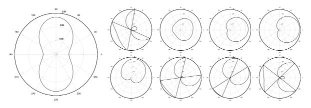
Figure 1: Directivity pattern and the eight phase patterns of the diversity array.
