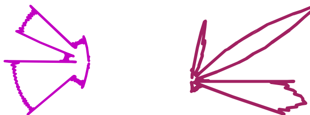
Multipath reception: selecting one beam or combining beams
