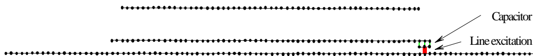
Figure 2. The FDTD grid pattern. The figure is a cross-section cut along the central y-directional line. The ground plane is only partially shown. The black lines represent y-directional PEC lines and the dots represent the x-directional PEC lines. The green lines represent the insulator in the capacitor, \epsilon_r = 30 , length of capacitor edge 2 mm. C = 1.1 \text{ pF} . The grid is 1 mm.
