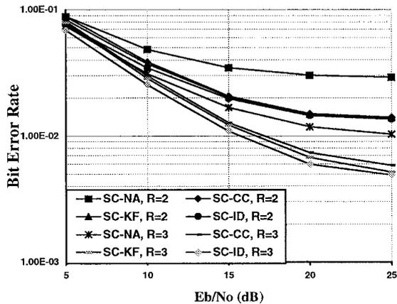
Fig. 3. BER performance of the SC-MAP equalizer (with  $R = 2$  and  $R = 3$ ) for the GSM-HT (Hilly Terrain) test channel @270.8 kb/s with  $L = 8$  taps, its power/delay profile being given in Table I. The fading spectrum is land-mobile with  $B_d = 10^{-4}/T_s$ , the modulation is BPSK (with no coding), the framing is (26, 58).
