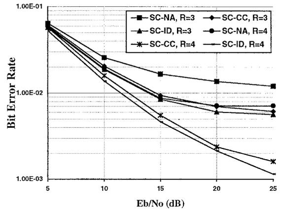
Fig. 5. BER performance of the SC-MAP equalizer (with  $R = 3$  and  $R = 4$ ) for the GSM-HT test channel @500 kb/s with  $L = 11$  taps, its power/delay profile being given in Table I. The fading spectrum is Land Mobile with  $B_d = 10^{-4}/T_s$ , the modulation is BPSK (with no coding), the framing is (52, 116).
