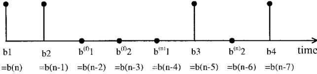
Fig. 1. Example of sparse channel of length  $L = 8$  with impulse response  $[1, 1, 0, 0, 0, 1, 0, 1]$  and positions of the  $R = 4$  nonzero symbols  $b(n) = [b_1 \ b_2 \ b_3 \ b_4]$ , the  $R_n = 2$  near hidden symbols  $b^{(n)}(n) = [b_1^{(n)} \ b_2^{(n)}]$  and the  $R_f = 2$  far hidden symbols  $b^{(f)}(n) = [b_1^{(f)} \ b_2^{(f)}]$ .
