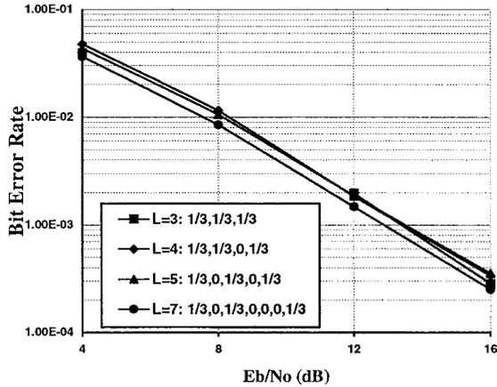
Fig. 2. BER performance of the SC-MAP equalizer for the reference WS-SUS channel constituted by  $R = 3$  independent Rayleigh-distributed nonzero taps with equal power, at different spacings. The different power/delay profiles are reported in the legenda. The fading spectrum is land-mobile with Doppler spread  $B_d = 10^{-4}/T_s$ , the modulation is BPSK (with no form of coding), the framing is (7, 18).
