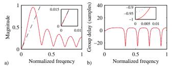
Fig. 7. a) Frequency response of the lattice second degree one-step-ahead PPFD of length N = 11 with coefficient word length of 8 bits (dotted) along with frequency responses of the corresponding unquantized (solid) and the optimum (dash-dot) differentiators. b) Group delay of the same filter with quantized (dotted) and exact (solid) coefficients.
