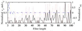
Fig. 3. Normalized magnitude response (solid), group delay (dotted) and noise gain (dash-dot) errors for the second degree PPFDs of lengths N = 3, ..., 100 with coefficients quantized to 16 bits.
