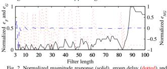
Fig. 2. Normalized magnitude response (solid), group delay (dotted) and noise gain (dash-dot) errors for the second degree PPFDs of lengths N = 3, ..., 100 with coefficients quantized to eight bits.
