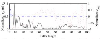
Fig. 5. Normalized magnitude response (solid), group delay (dotted) and noise gain (dash-dot) errors of the second degree lattice PPFDs of lengths N = 3, ..., 100 with coefficients quantized to eight bits.
