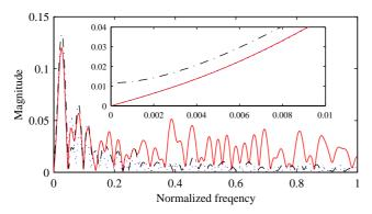
Fig. 3. Frequency response of the solution found for N = 80 with  $(P_{M}, P_{co}) = (0.1/N, 0.8)$  after 181 generations (run 3 in Table 1) (solid). Also shown are the frequency response of the exact coefficient filter given by (7) for N = 80 (dotted), and of the same filter with the coefficients quantized to 8 bits (dash-dot).
