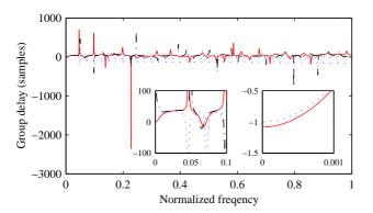
Fig. 4. Group delays of the filters shown in Fig. 3; genetic solution (solid), exact coefficient filter (dotted), and the exact coefficient filter after coefficient quantization to 8 bits (dash-dot).
