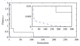
Fig. 2. Fitness (8) of the best solution in each generation over one run for filter length N = 80 with each of the parameters (12);  $(P_{_{MP}}, P_{_{CO}}) = (0.1/N, 0.8)$ , run 3 (solid),  $(P_{_{MP}}, P_{_{CO}}) = (1/N, 0.4)$ , run 2 (dotted), and  $(P_{_{MP}}, P_{_{CO}}) = (4/N, 0.1)$ , run 1 (dash-dot).
