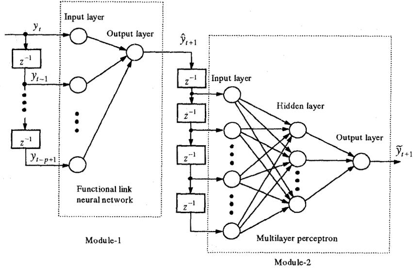
Fig. 1. The structure of the hybrid neural network-based predictor.
