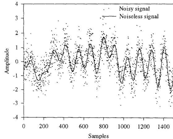
Fig. 4. Noisy and noiseless in-phase component of power signal at 5 km/h using Jakes' model.
