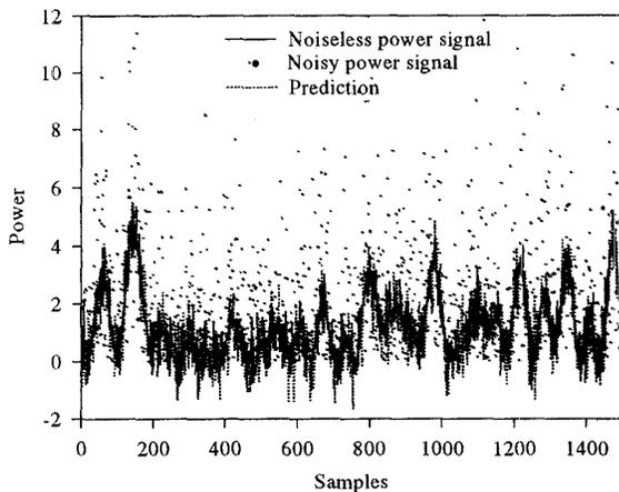
Fig. 6. Noisy and noiseless power signals, and the prediction of the optimal neural predictor under the component SNR of 0 dB.
