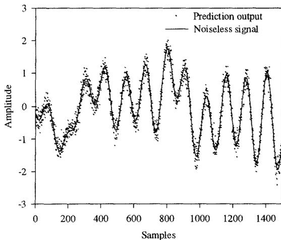
Fig. 5. The prediction of noisy in-phase component of power signal under 0 dB at 5 km/h.
