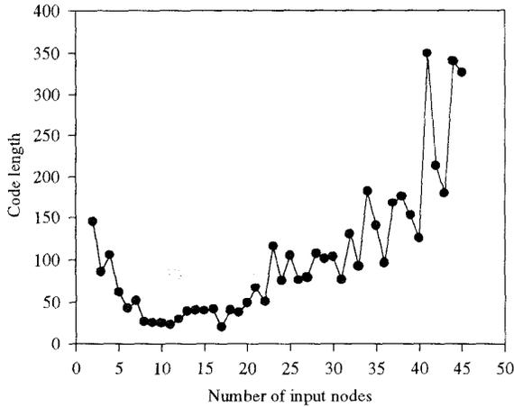
Fig. 2. Code lengths of different models of FLNN under component SNR = 0 dB.
