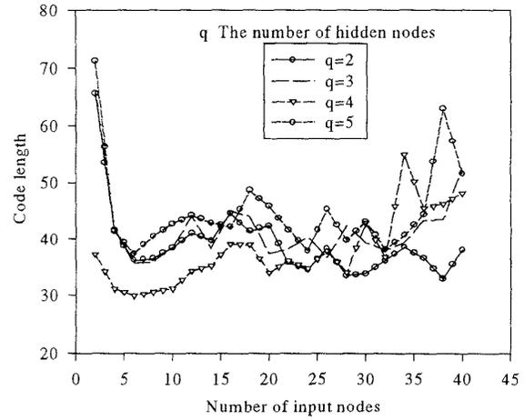
Fig. 3. Code lengths of different models of MLP under component SNR = 0 dB.
