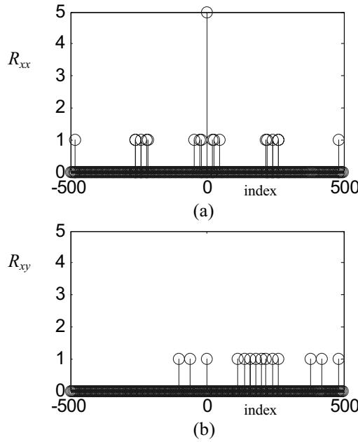
**Fig. 3** Correlation amplitude (a) autocorrelation of a low rate code (b) cross-correlation between a low rate and a high rate codes.
