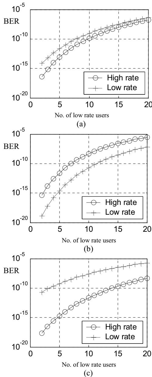
**Fig. 4** BER for the class OOC high rate and low rate classes with  $K_{HR} = 4$  and (a)  $W_{HR} = 5$ ,  $W_{LR} = 5$  (b)  $W_{HR} = 5$ ,  $W_{LR} = 7$  (c)  $W_{HR} = 7$ ,  $W_{LR} = 5$ .
