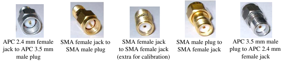
Figure 6.1: Adapters used with a network analyzer for measurements and calibration of the device itself.
