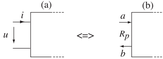
Figure 6.1: Definition of (a) K- and (b) W-variables at a port of a circuit element.
