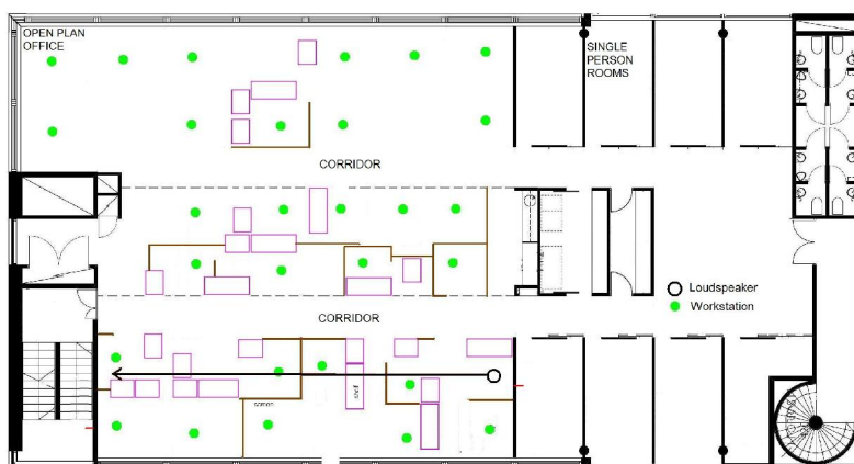
Figure 1. An example of measurement line (arrow) in an open office. Furniture layout is outlined only in the area of measurement. The line should locate close to workstations. The measurements are, always, carried out in the workstations.
